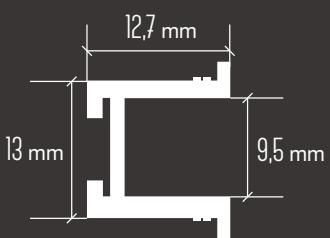
Corpus slide rail made of plastic has to be clipped into the aluminium profile (order separately).
